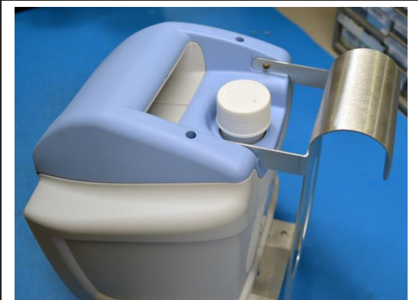
Step 10: Replace the reservoir cap.
