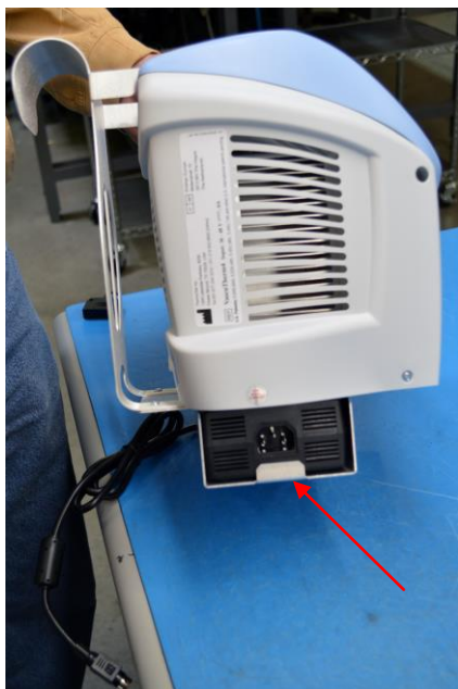
Step 12a: Continue to slide the power supply until it meets the bracket stop.
