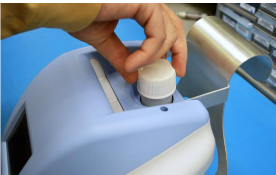
Step 8: Unscrew and remove the reservoir cap.
