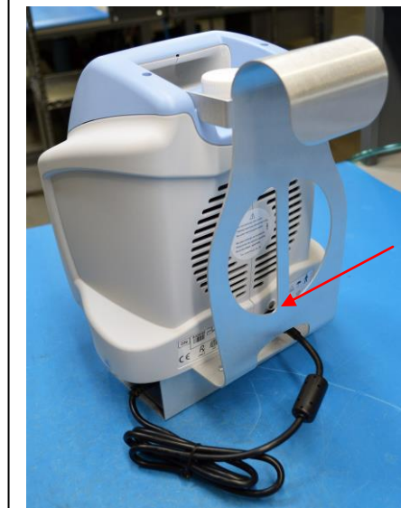
Step 13: Plug in the power supply to the appropriate port on the back of the unit.
