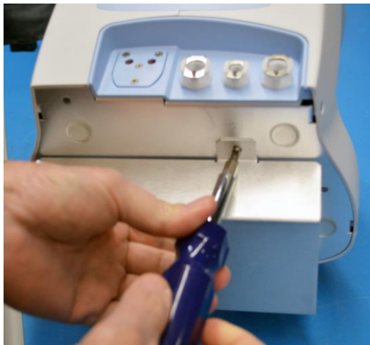
Step 11: Secure the bracket to the bottom of the unit by replacing the screw previously removed.
