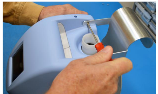
Step 9: Install (2) M3x6 Phillips flat screws to secure the bed hook to the top of the unit.
