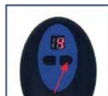
Power off by pressing down on the "OFF" button for 5 seconds. Reference the User Manual for warnings and product specifications.
